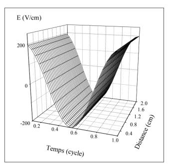
Figure 3.1: Temporal and spatial variations of the electric field for the first cycle.
