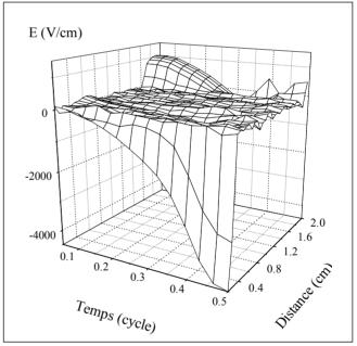
Figure 4.2: Temporal and spatial variations of the electric field for the third cycle.
