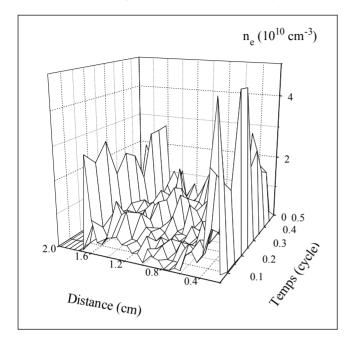
**Figure 5.1:** Temporal and spatial variations of the electron density for the third rf cycle.
