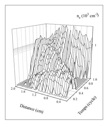
Figure 3.3: Temporal and spatial variations of the electron density for the first rf cycle.
