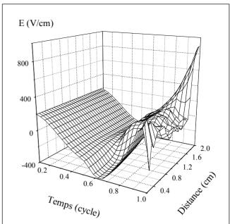
Figure 4.1: Temporal and spatial variations of the electric field for the second cycle.
