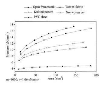
Figure 4: P-A curve predicted from the Steel-Polymers contact.
