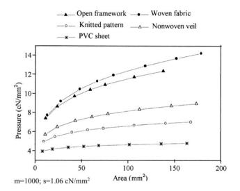
Figure 3: P-A curve predicted from the Poly(methyl Metacrylate)-Polymers contact.
