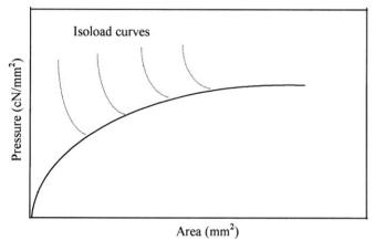
Figure 1: Generalized Pressure-Area Deformation Curve.
