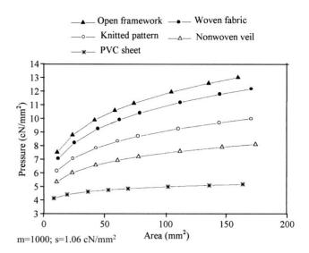
Figure 2: P-A curve predicted from the Aluminium-Polymers contact.
