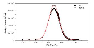
**Figure 12:** Density of states versus (Et-Ev). Full squares td = 220s, triangular td = 85 s. Full and broken curves
