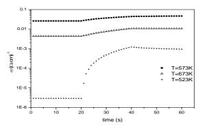
**Figure 9:** Photoconductivity versus time of undoped ZnO films. (Effect of substrate temperature).
