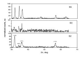
Figure 1: X-rays diffraction spectra (effect of substrate temperatureTs).
