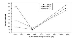
Figure 3 : Texture coefficient versus temperature Ts.
