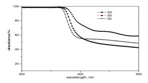
Figure 4: Absoption spectra (substrate temparature effect), td =220s.
