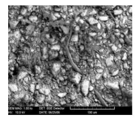
Figure 5 : SEM Micrograph of fractured surface showing the presence of inclusions.
