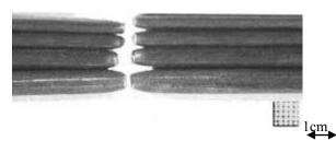
Figure 2 : Optical micrograph showing the ductile failure of the material.
