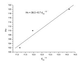
Figure 7: Hardness of recrystallized material versus d<sub>rec</sub><sup>-1/2</sup>
