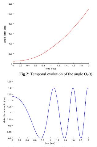
Fig.3: Temporal evolution of the slider displacement x(t).
