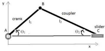
Fig.1: Slider-crank mechanism
