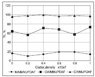
**Figure 7:** Track loss clutter density for manoeuvring targets, with a minimum separation distance equal to 800 m, using MAIMMJPDAF, OAIMMJPDAF and CIMMJPDAF with a mean update time equal to 2.8s.
