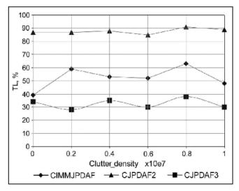
Figure 4: Track loss rate vs. clutter density for manoeuvring targets, with a minimum separation distance equal to 800m, using
