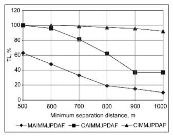
**Figure 8:** Track loss rate vs. Minimum separation distance for manoeuvring targets, in clutter with a density  $\lambda = 0.6 \times 10^{-6}$ , using MAIMMJPDAF, OAIMMJPDAF and CIMMJPDAF with a mean update time equal to 2.8s.
