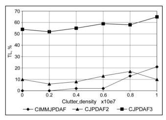
**Figure 3:** Track loss rate vs. clutter density for crossing targets, with a 10 degrees crossing angle, using CIMMJPDAF,CJPDAF3 and CJPDAF2 with a constant update time equal to 1.5s.
