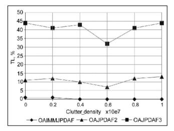
**Figure 5:** Track loss rate vs. clutter density for crossing targets, with a 10 degree crossing angle, using OAIMMJPDAF, OAJPDAF3 and OAJPDAF2 with a mean update time equal to 1.5s.
