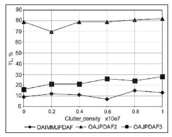
Figure 6: Track loss rate vs. clutter density for manoeuvring targets, with a minimum separation distance equal to 800m, using OAIMMJPDAF, OAJPDAF2 and OAJPDAF3 with a mean update time equal to 1.5s.
