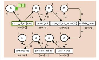
Figure 8 : A CPN corresponding to the *RegularGeneration* scenario.
