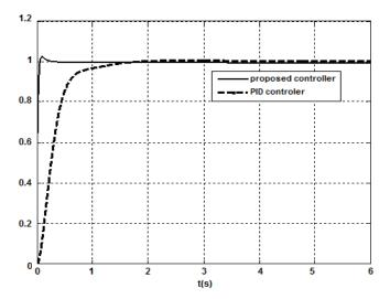
Figure <u>10</u>: The terminal voltage step response of the closed loop AVR system with the PID controller and with the proposed controller for Kg = 0.7 and  $\tau_g = 1$  s
