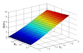
Figure 15 : Plot of the overshoot Os(%) versus  $K_g$  and  $\tau_g$  of the AVR system with a classical PID controller of [25]
