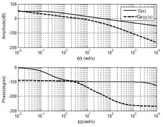
**Figure 7**: Bode plots of the open loop transfer functions G(s) and  $G_{PID}(s)$
