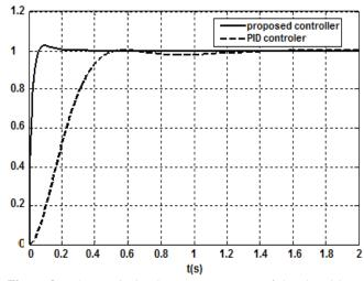
**Figure 8** : The terminal voltage step response of the closed loop AVR system with the proposed controller and with the PID controller
