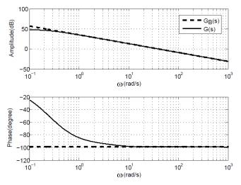
**<u>Figure 4</u>**: Bode plots of the open loop function G(s) and the Bode's ideal function  $G_B(s)$
