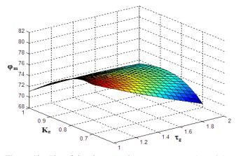
**<u>Figure 13</u>**: Plot of the phase margin  $\phi_m$  versus  $K_g$  and  $\tau_g$  of the AVR system with a classical PID controller of [25]
