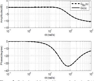
Figure 5: Bode plots of the closed loop transfer function  $G_c(s)$  and the ideal closed loop transfer function  $G_{Bc}(s)$
