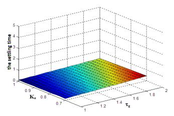
Figure 16 : Plot of the settling time versus  $K_g$  and  $\tau_g$  of the AVR system with the proposed controller
