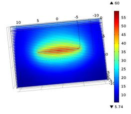
Figure 9 : Temperature distribution around the GHX
