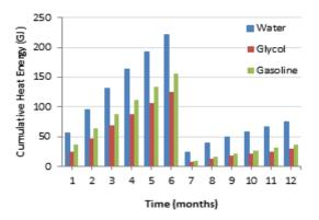
Figure 13 : Cumulative heat stored and recovered for the fluid carrier sensitivities
