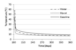
Figure 12 :1 Temperature of the fluid carrier at the outlet of the GHX
