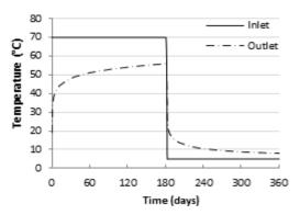
Figure 8 : Fluid carrier temperature at the inlet and outlet of the GHX
