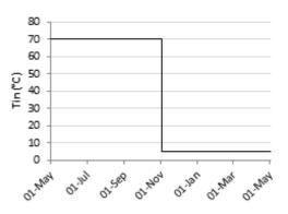
Figure 3 : Temperature of the working fluid at the duct inlet
