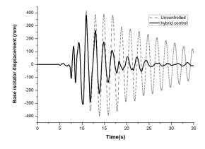
Figure 4: Base displacement under Kobe earthquake
