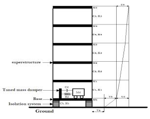
Figure 1: Base-isolated structure with tuned mass damper
