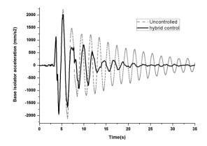
Figure 9: Base acceleration under Northridge earthquake
