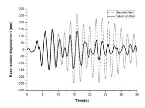
Figure 3: Base displacement under Hachinohe earthquake
