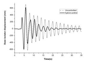
Figure 5: Base displacement under Northridge earthquake
