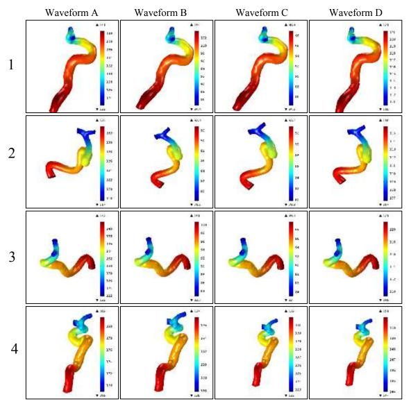
**Figure 5**. Pressure distribution inside the ICAs (1), (2), (3) and (4) after CFD simulation using the four-inlet waveforms boundary condition.
