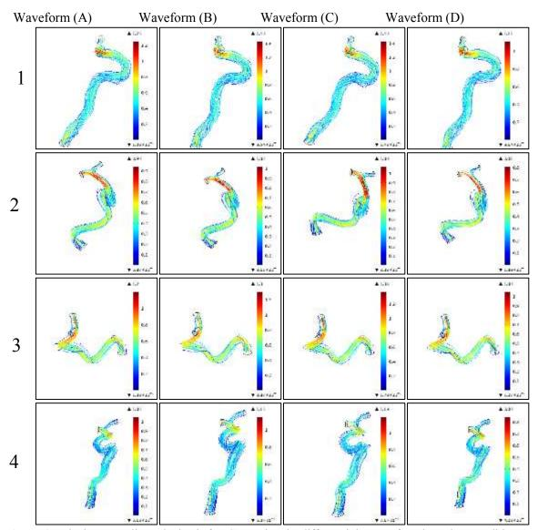
Figure 6. Velocity streamlines obtained after CFD using the different inlet waveform boundary condition applied.
