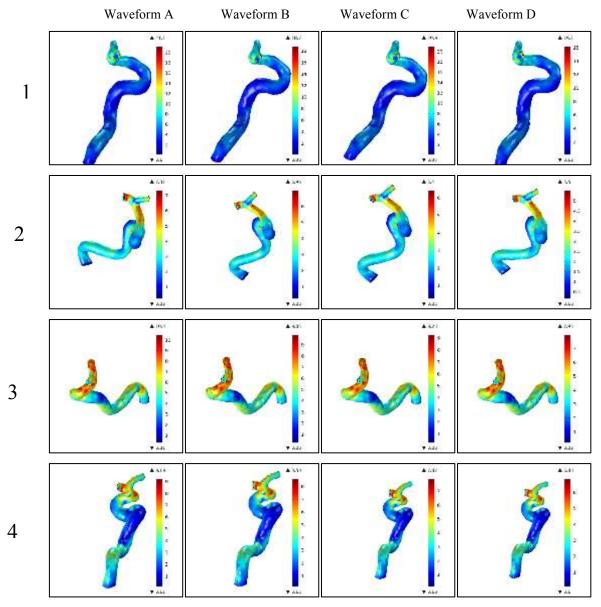
Figure 2. WSS distributions at the four ICAs (1), (2), (3) and (4) from pulsatile flow simulations using the four different waveforms (A), (B), (C) and (D) using the same mean inflow boundaries conditions.
