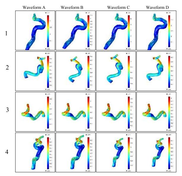
Figure 4. TAWSS distribution after the application of the four inlet waveform boundaries conditions to the CFD.
