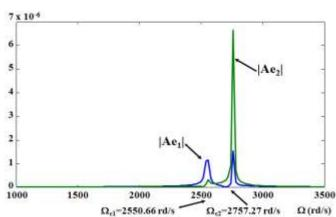
Figure 8(a): Response to an asynchronous force: rotor with one disc free-simply supported case.
