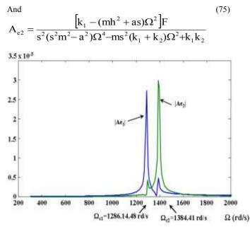
Figure 6(a) : Response to a synchronous force: rotor with one disc, free-simply supported case.
