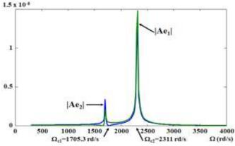
**Figure 8(c)**: Response to an asynchronous force: rotor with three discs free-simply supported case.
