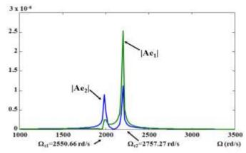
**Figure 8(b)**: Response to an asynchronous force: rotor with two discs free-simply supported case.
