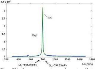
Figure 5(b): Response to a synchronous force: rotor with two discs, simply-simply supported case
