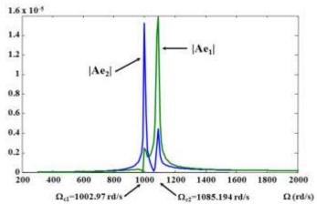
**Figure 6(b)** : Response to a synchronous force: rotor with two discs free-simply supported case.
