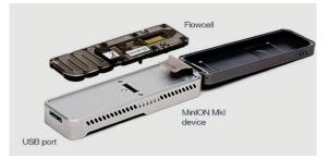
Figure 1: MinIon device (from oxford nanopore technologies).
