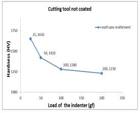
Figure 4: Hardness of the uncoated cutting tool
