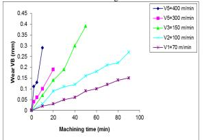
Figure 7: Combinations of different wear curves for W-TIN coated cutting tools
