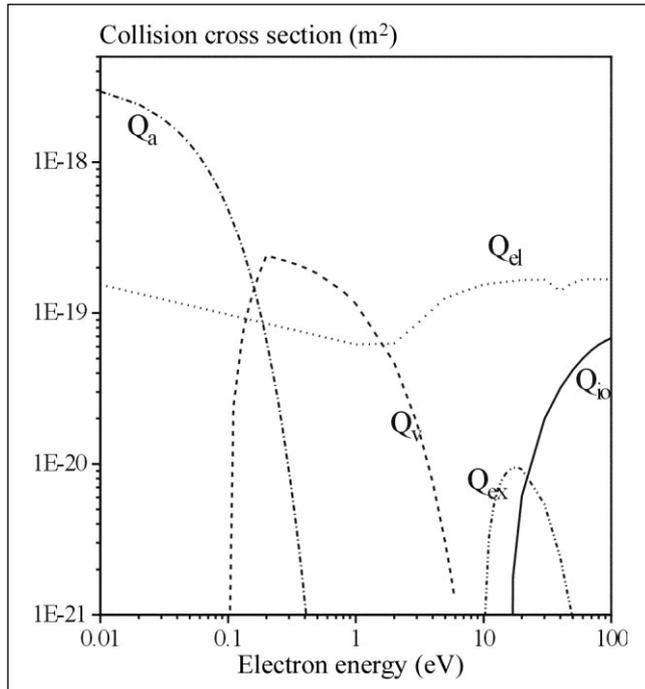
**Figure 2:** Summary of collisional cross section of SF<sub>6</sub>:  $Q_{el}$ : elastic momentum transfer cross section;  $Q_{At}$ : attachment,  $Q_{ex}$ : electronic excitation,  $Q_v$ : vibrations, and  $Q_{ion}$ : ionization .
