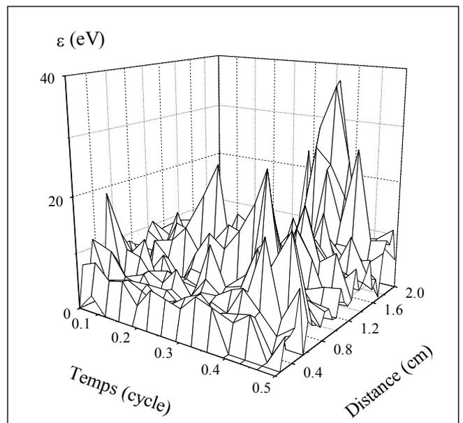
**Figure 6:** Temporal and spatial variations of the mean energy of electrons for the third rf cycle.
