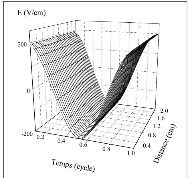
**Figure 3.1:** Temporal and spatial variations of the electric field for the first cycle.
