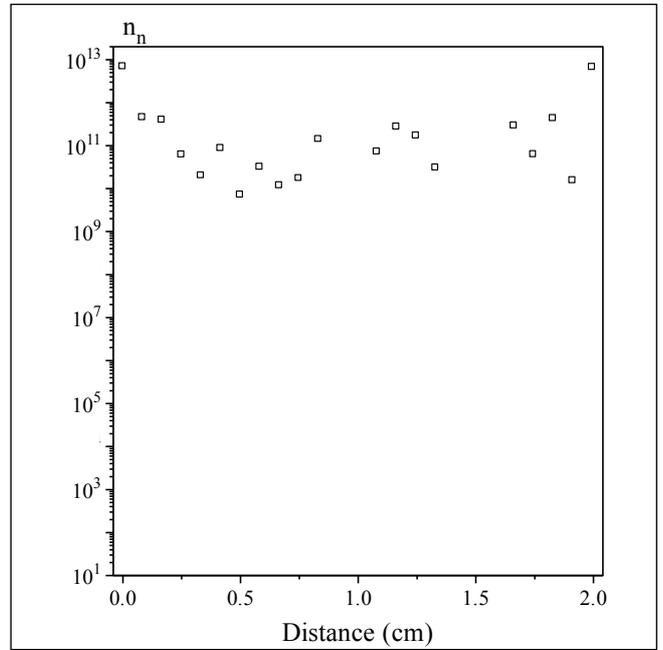
**Figure 5.3:** Spatial variations of the negative ion distribution ( $n_n$  should be multiplied by 0.04 to convert to densities  $\text{cm}^{-3}$ ).
