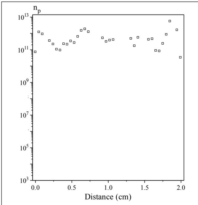
**Figure 5.2:** Spatial variations of the positive ion distribution ( $n_p$  should be multiplied by 0.04 to convert to densities  $\text{cm}^{-3}$ ).
