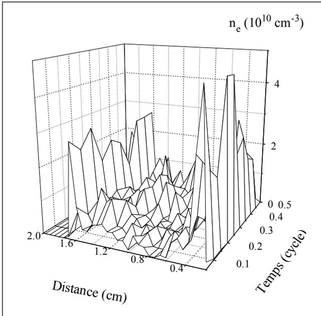
**Figure 5.1:** Temporal and spatial variations of the electron density for the third rf cycle.
