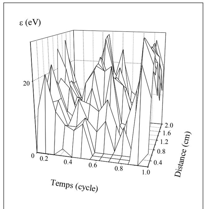
**Figure 3.2:** Temporal and spatial variations of the mean energy of electrons for the first rf cycle.
