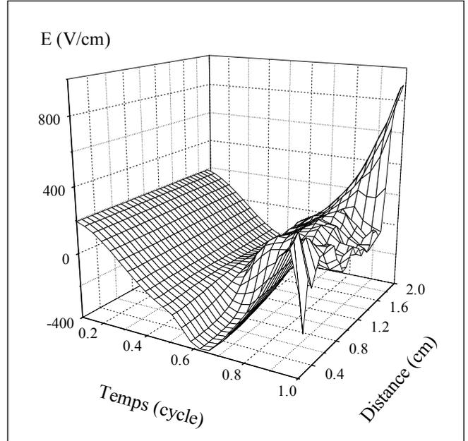
**Figure 4.1:** Temporal and spatial variations of the electric field for the second cycle.
