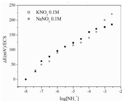
**Fig.1.** Output voltage of ammonium –ISFET vs. log  $[\text{NH}_4^+]$  in  $\text{KNO}_3$  0.1 M and  $\text{NaNO}_3$  0.1 M.
