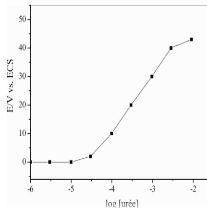
**Fig .2 .** Potentiometric response of urea biosensors using 5mM phosphate buffer to urea concentration increase .
