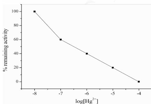
**Fig. 3** . Dependence of remaining activity of the biosensors on the concentration of the inhibitor metal ion Hg (II).
