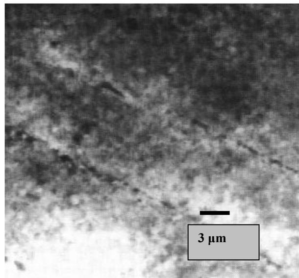
**Figure 6:**  $Al_6Mn$  precipitates
