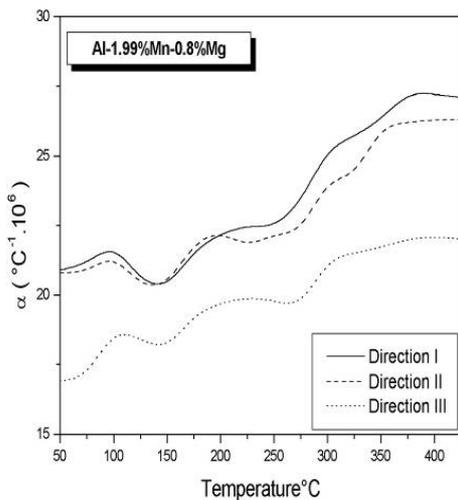
**Figure 5:** Variation of the thermal expansion coefficient  $\alpha$  (T) of
