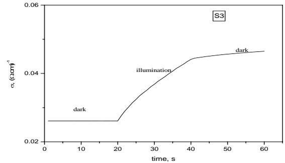
**Figure 10:** Photoconductivity versus time.
