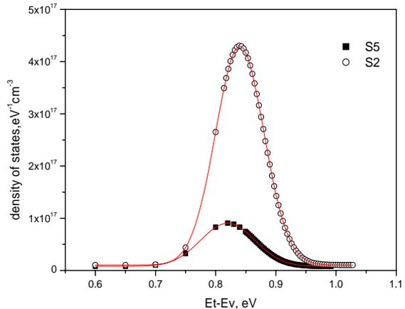
**Figure 13.** Density of states versus  $(E_t - E_v)$ .
