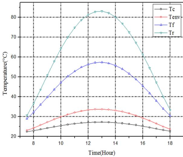
Figure.3 Temperature components of the collector
