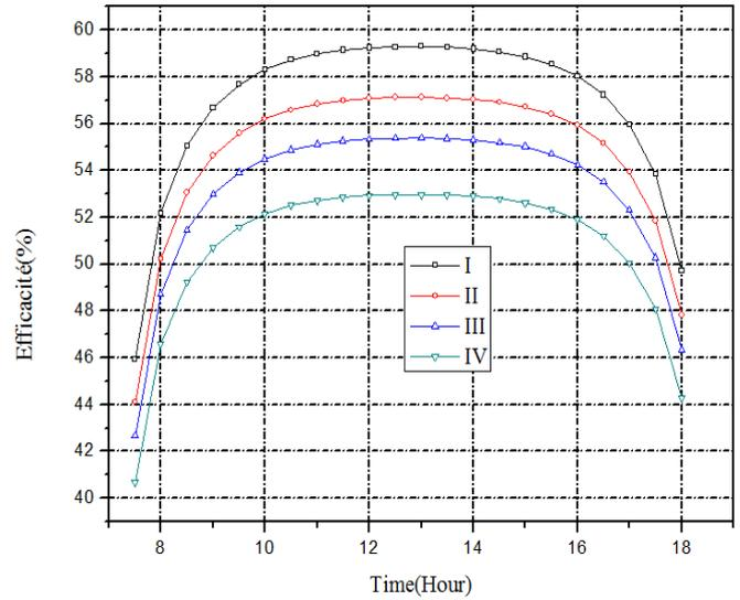
Figure.9 Effect of the ratio of concentration on daily variation of efficiency (I=2, II=1.5, III=1.25, IV=1)
