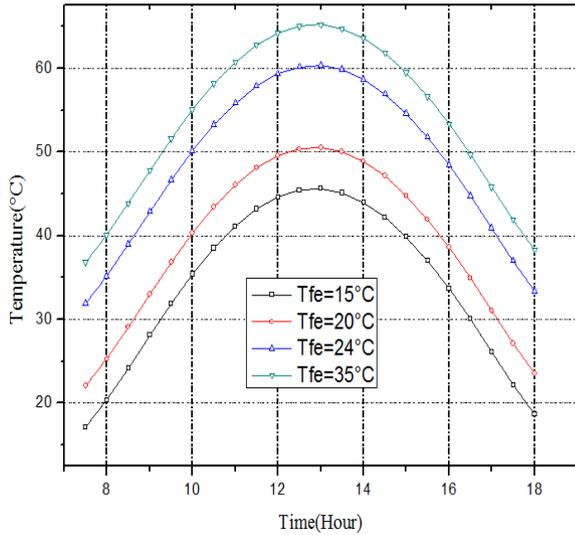
Figure.7 Effect the inlet temperature on the average temperature of fluid
