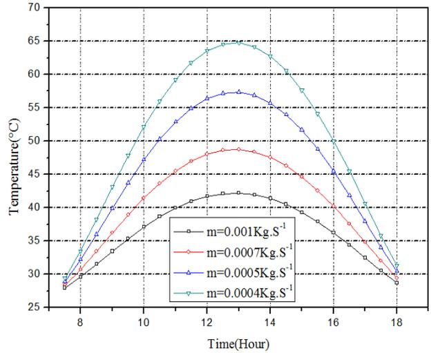
Figure.5 Effect the mass flow on fluid temperature
