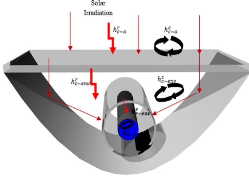
Figure 2 Presentation of heat exchange on the collector
