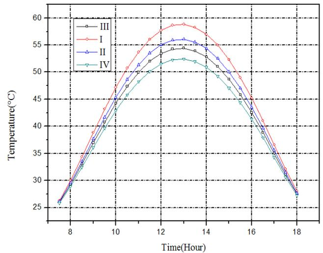
Figure.10 Effect the ratio of concentration on daily variation of fluid temperature (I=2, II=1.5, III=1.35, IV=1.5)
