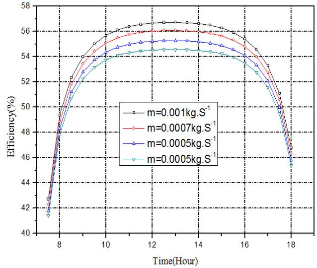
Figure.6 Effect the mass flow on the efficiency of the collector
