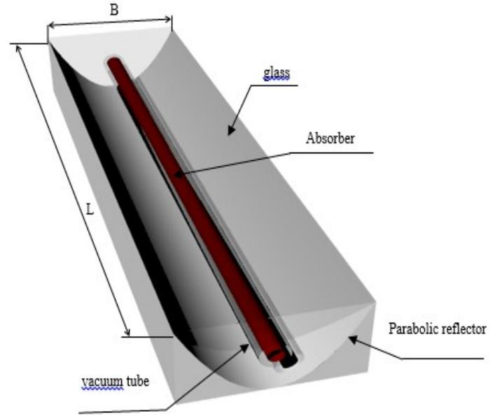
Figure. solar collector
