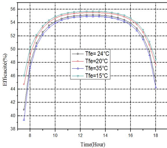
Figure.8 Effect the inlet temperature on the collector efficiency
