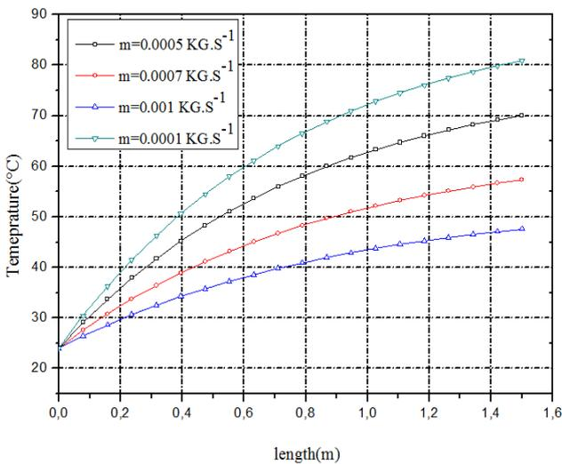
Figure.4 Effect the mass flow on the local temperature in the direction of the flow
