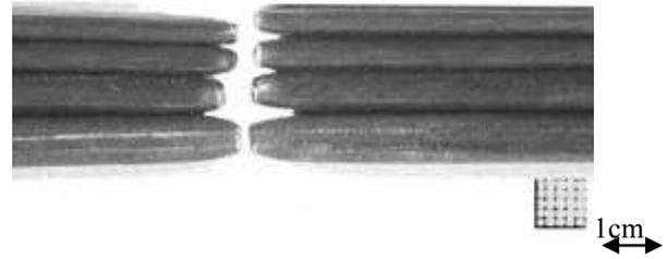
Figure 2 : Optical micrograph showing the ductile failure of the material.
