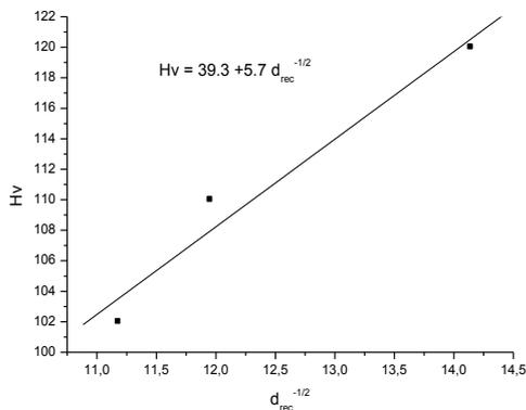
Figure 7: Hardness of recrystallized material versus  $d_{rec}^{-1/2}$
