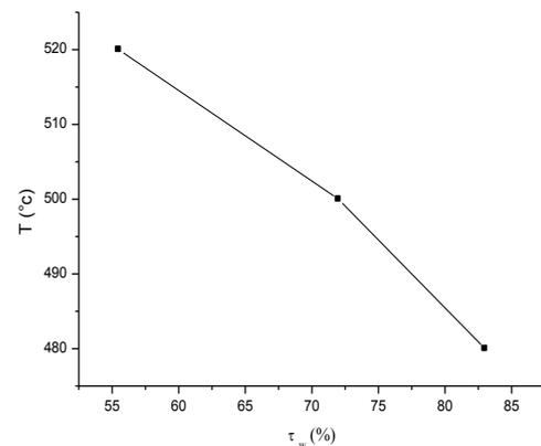
Figure 6 :Total recrystallisation temperature as a function of area reduction  $\tau_w$ .
