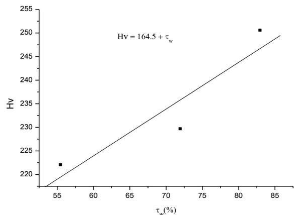
Figure 3 : Hardness as a function of  $\tau_w$  in as received conditions
