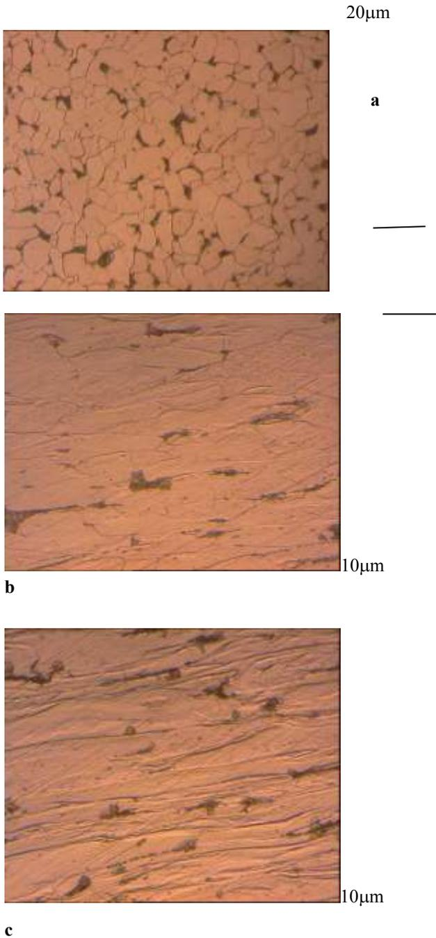
Figure 1 : Optical micrographs of the material in as received conditions: a)  $\phi = 6\text{mm}$ , b)  $\phi = 3.18\text{mm}$ , c)  $\phi = 2.45\text{mm}$ .
