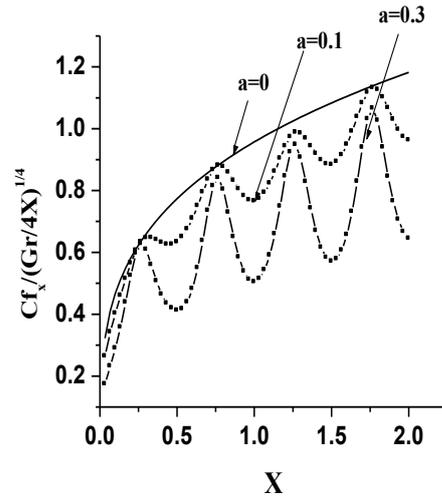
Fig.5 Skin-friction coefficient for different values of the amplitude wavelength and for m=0
