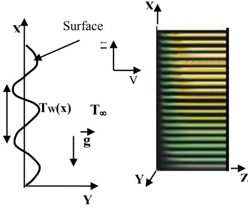
Fig.1 Physical model and coordinates system
