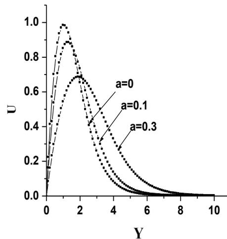
Fig.2.a Velocity profiles at X=0.5 for different values of the amplitude wavelength and for m=0
