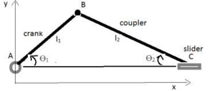
Fig.1: Slider-crank mechanism
