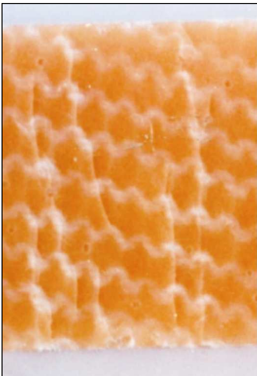
Figure 7: Fissuration transverse (agrandissement x 8).
