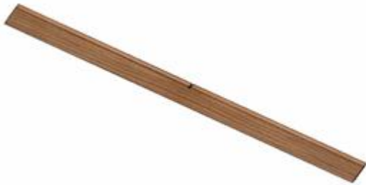
Figure 1 : Standard specimen of Charpy Impact test
