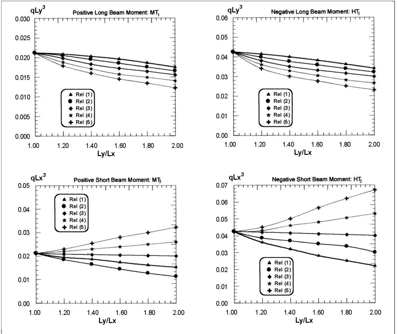
**Figure 5:** Effects of the panel shape and the ratio  $I_1/I_2$  on the twistless behaviour of a internal slab-beam system.
