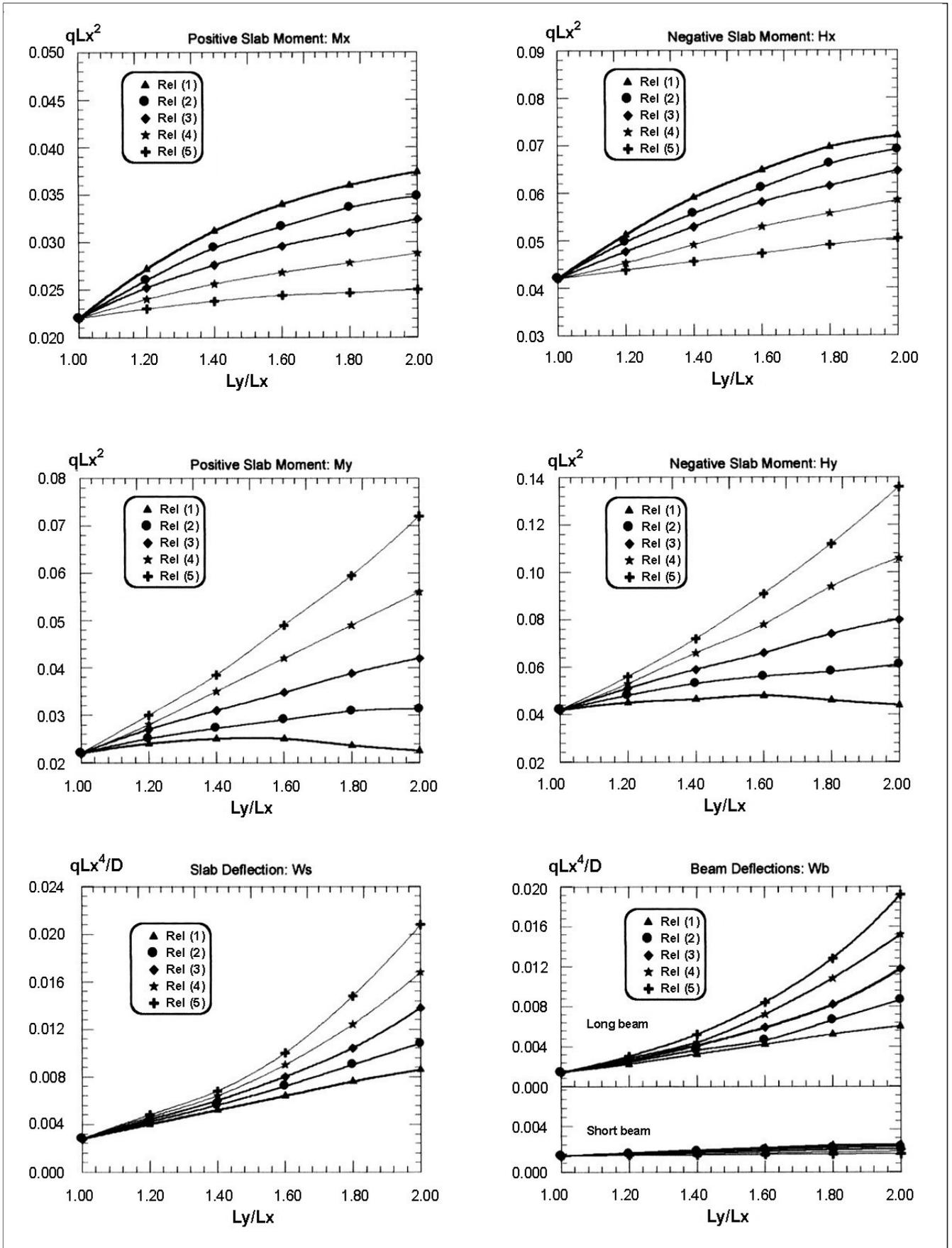
**Figure 4:** Effects of the panel shape and the ratio  $I_1/I_2$  on the twistless behaviour of an internal slab-beam system.
