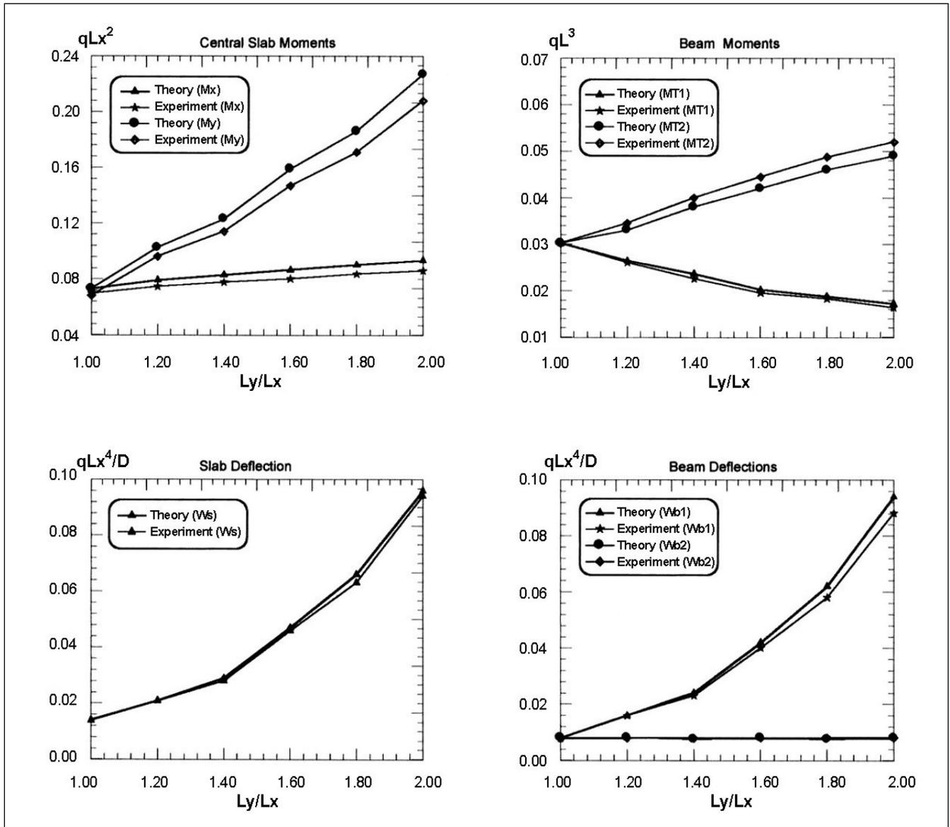
**Figure 9:** Theoretical and experimental results of a single slab-beam system with various panel shapes.
