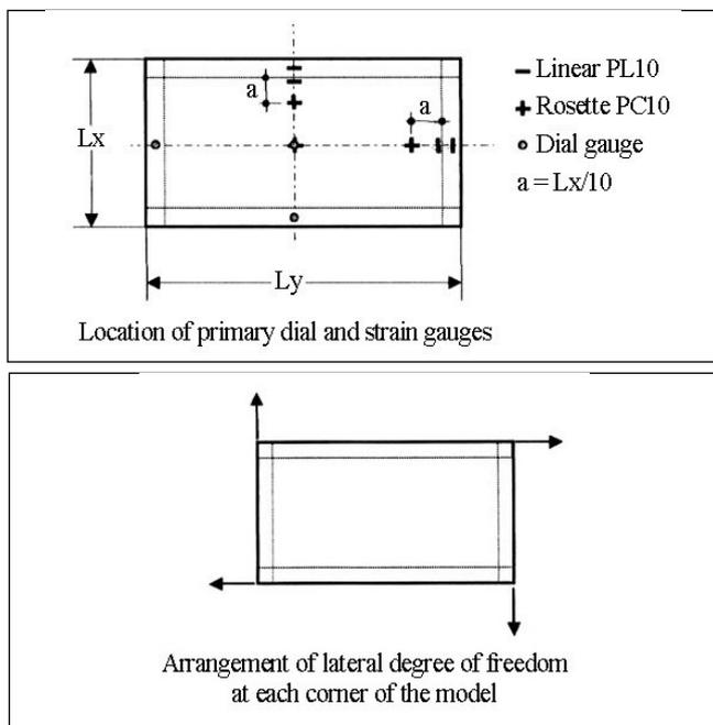
Figure 7: Single slab-beam model.
