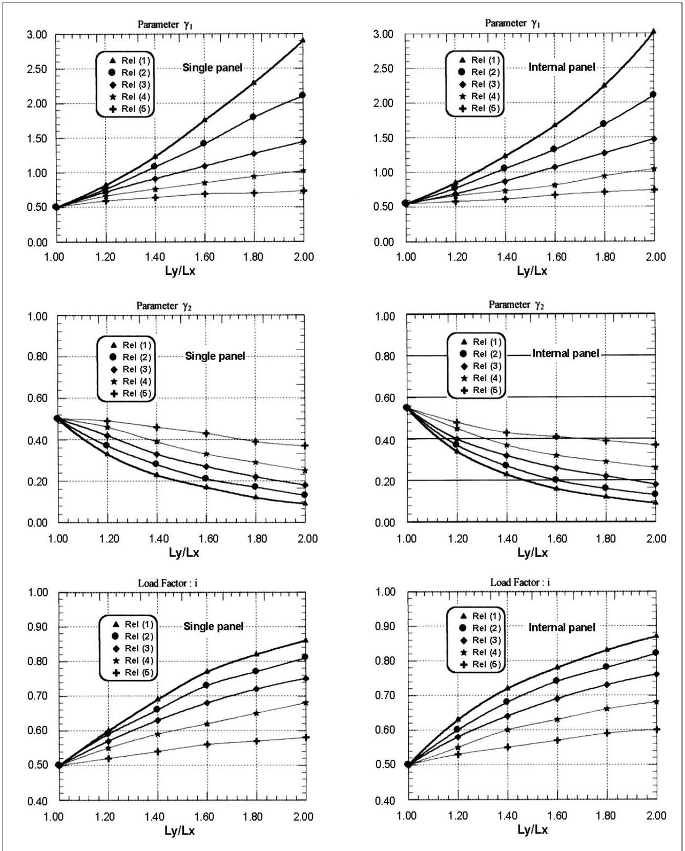
**Figure 6:** Beam/slab stiffness ratios and load distribution factors for twistless behaviour in slab-beam systems.
