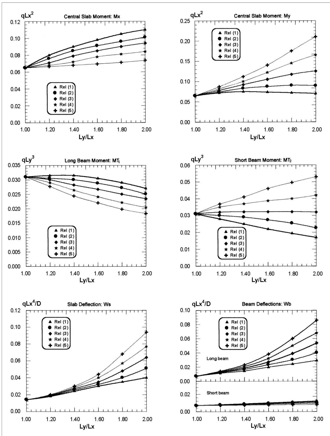
**Figure 3:** Effects of the panel shape and the ratio  $I_1/I_2$  on the twistless behaviour of a single slab-beam system.
