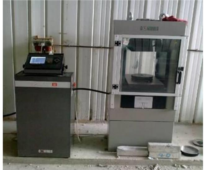
**Figure 1** : Compression testing machine
