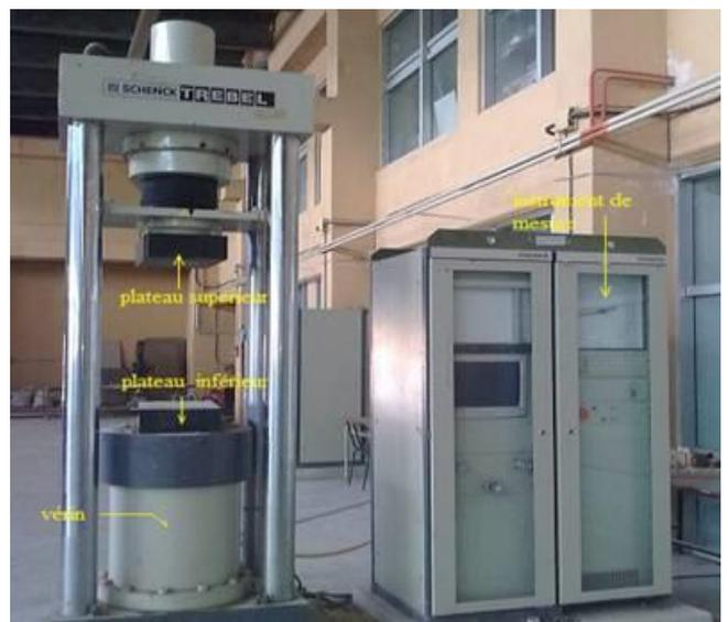
**Figure 2** : Bending testing machine
