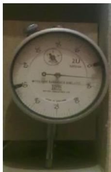
**Figure 5 :** Comparator displacement device
