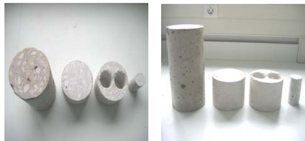
Figure 1 : Confection des mini-cylindres 4x8cm
