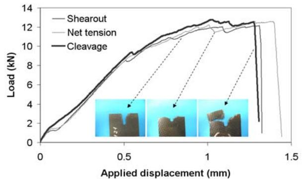
**Figure 8** : Load-displacement curves and associated fracture mode for a bearing test on a  $[0/45/45/0]_S$  carbon/epoxy laminate for  $W/D=8$ .
