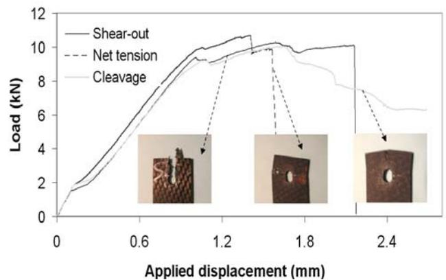
**Figure 11** : Load-displacement curves and associated fracture mode for a single lap bolted joint test on a [0/45/45/0]<sub>s</sub> carbon/epoxy laminate for W/D=5
