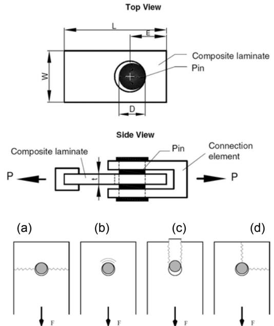
**Figure 7** : Configuration of a single-bolt double lap bolted joint test on composite laminates and corresponding macroscopic failure modes [14]
