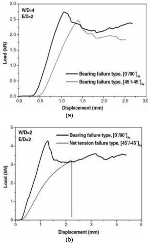
**Figure 9** : Load-displacement curves for carbon/PPS UD laminates with different W/D ratios :
