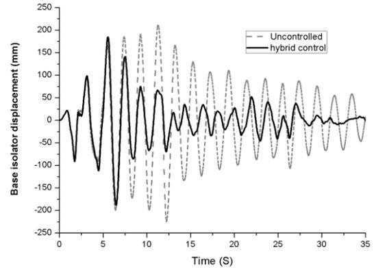
**Figure 2 :** Base displacement under El Centro earthquake
