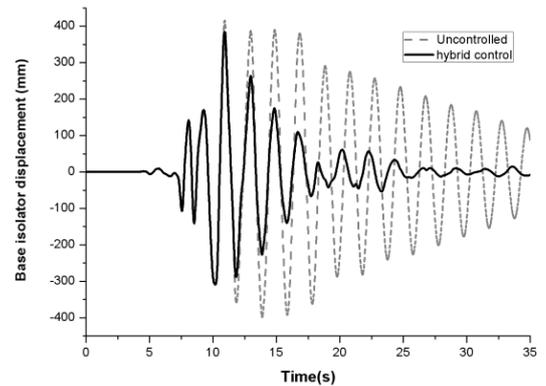
**Figure 4 :** Base displacement under Kobe earthquake
