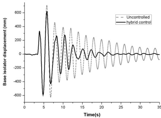
**Figure 5 :** Base displacement under Northridge earthquake
