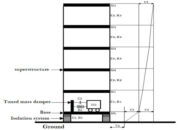
Figure 1 : Base-isolated structure with tuned mass damper
