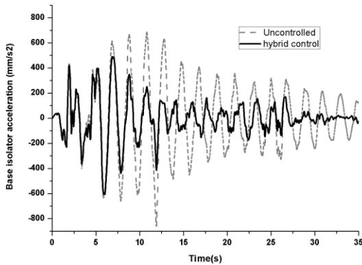
**Figure 6 :** Base acceleration under El Centro earthquake
