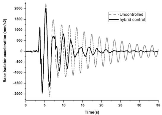
**Figure 9 :** Base acceleration under Northridge earthquake
