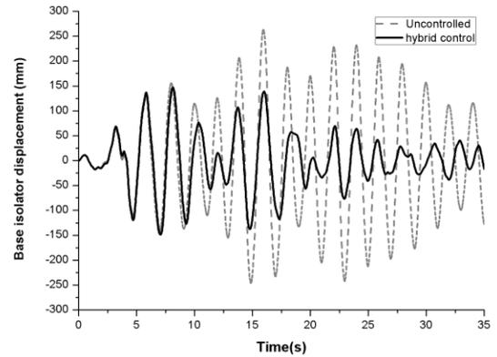
**Figure 3 :** Base displacement under Hachinohe earthquake
