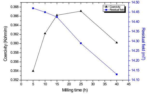
Fig.5. illustrates the evolution of the coercivity and lattice parameters versus milling time. The evolution of the coercivity increases in the same way of the curve representing the lattice parameter. As for soft magnetic systems in general, the coercivity of FeCo alloys depends strongly on the microstructure.
