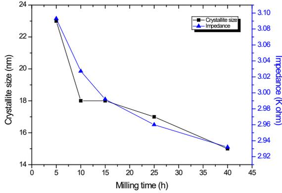
The evolution of the impedance (Z) and crystallite size versus milling time at 4862Hz frequency follows the same evolution, Fig. 2.
