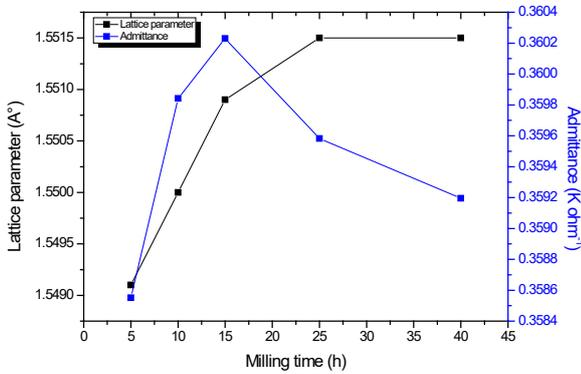
Fig.3. illustrates the evolution of the admittance and lattice parameters versus milling time in low frequency. The evolution of the admittance increases in the same way of the curve representing the Lattice parameter. The evolution of the admittance and lattice parameter versus milling time at 1000Hz frequency has the same evolution, Fig. 3.
