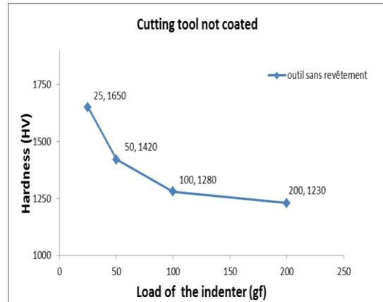
Figure 4: Hardness of the uncoated cutting tool
