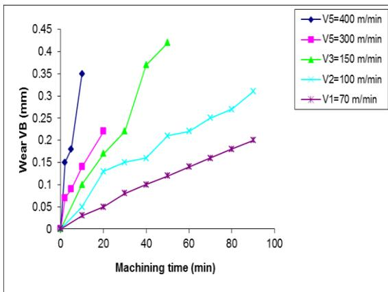
**Figure 6:** Combinations of the different wear curves for uncoated cutting tools.
