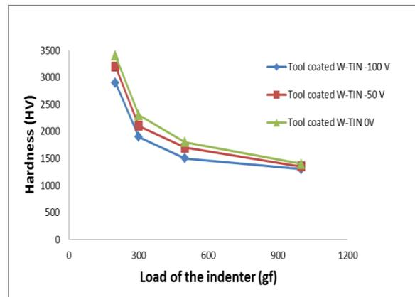
Figure 5: Hardness of cutting tools coated by W-TIN
