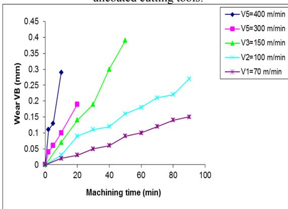
**Figure 7:** Combinations of different wear curves for W-TIN coated cutting tools
