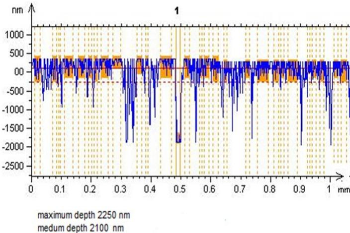
Figure 2: Measurement of the thickness of the deposited layer.
