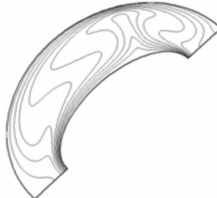
FIG. 8 Isotherms for  $e_1=0.86$ ,  $Fr=5$ , and  $Gr=5.10^4$   $\alpha=45^\circ$
