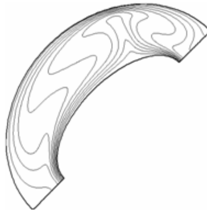
FIG. 8 Isotherms for e_1=0.86 , Fr=5 , \alpha=45^\circ and Gr=5.10^4
